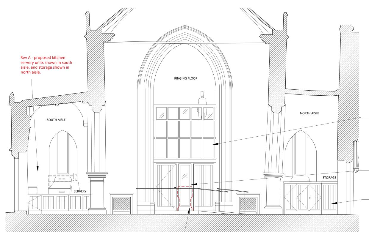
Balustrade to ringing chamber and upper section of decorative screen above doors to be replaced with timber framed panelled screen with glazed inserts at upper level, in style to match proposed glazed screen to meeting room in north aisle.
